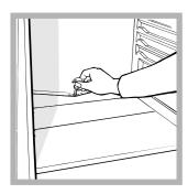
The refrigerator has an automatic defrosting function: water is ducted to the back of the appliance by a special discharge outlet (see diagram) where the heat produced by the compressor causes it to evaporate.
